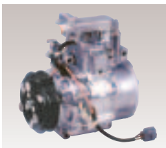
■ Hybrid-Type Compressors Designed to meet the needs of hybrid vehicles. These units are compact and lightweight and adopt DC brushless motors with high-performance neodymium magnets and realize sophisticated control through the application of control computers.
