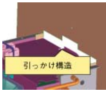
Fixation of the fan duct and air duct
