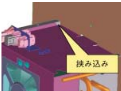
Fixation of the fan duct and evaporator
